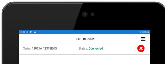
Once a device has been paired, the serial number and status will be displayed below the title bar. A paired device can be disconnected by tapping the [✖] icon.
