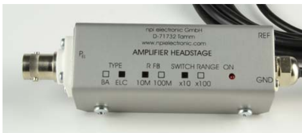
Figure 9: ELC x10 / x100 switchable headstage
