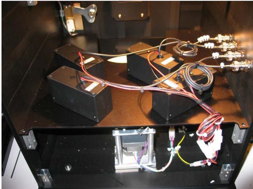
Plug the 4 power connectors into their mating connectors underneath the PMT plate. It does not matter which one goes to which connector. They are all equivalent. Make sure the wires hang so that they are not near the turntable.
