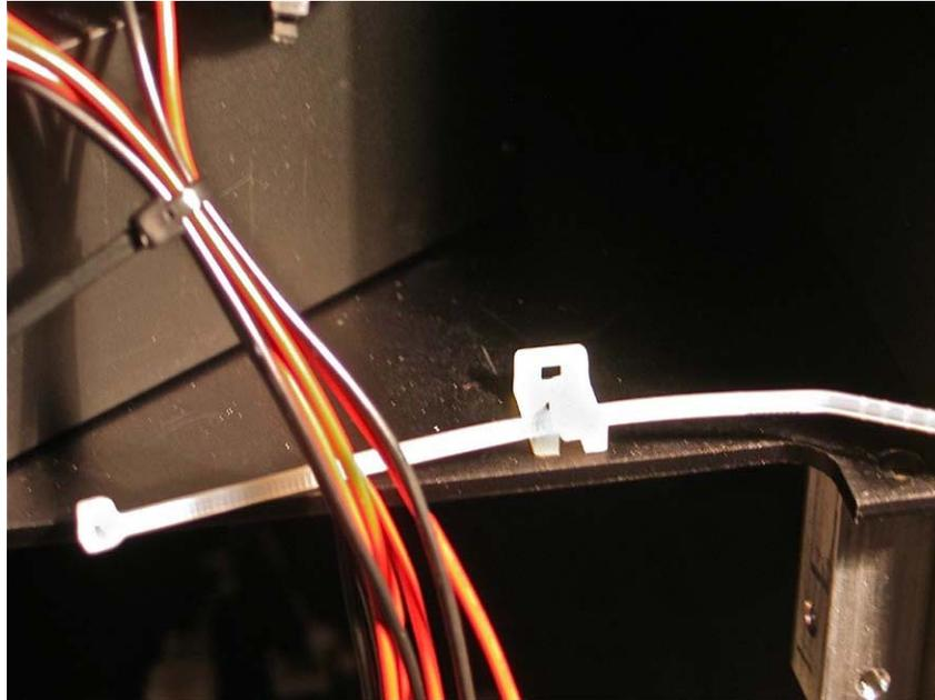
Connect the front two PMT's signal (BNC cables). First coil up the excess from each into a 5 cm coil (see photos), place a couple of cable ties on the coil, and then plug the connectors in to the front two BNC connectors (A to 1, B to 2). The cable ties should be snug, but not tight.
